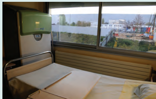
The mobile Plasmair unit (above, left) is used to remove/inactivate airborne particles from the rooms of neutropenic cancer patients at Dijon Hospital.
